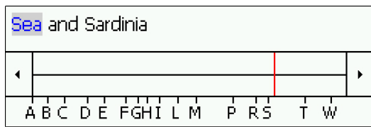
Figure 3. The Alphasl原因 redesign to speed up user interaction. Dragging operations can be initiated anywhere on the slider tiles.
